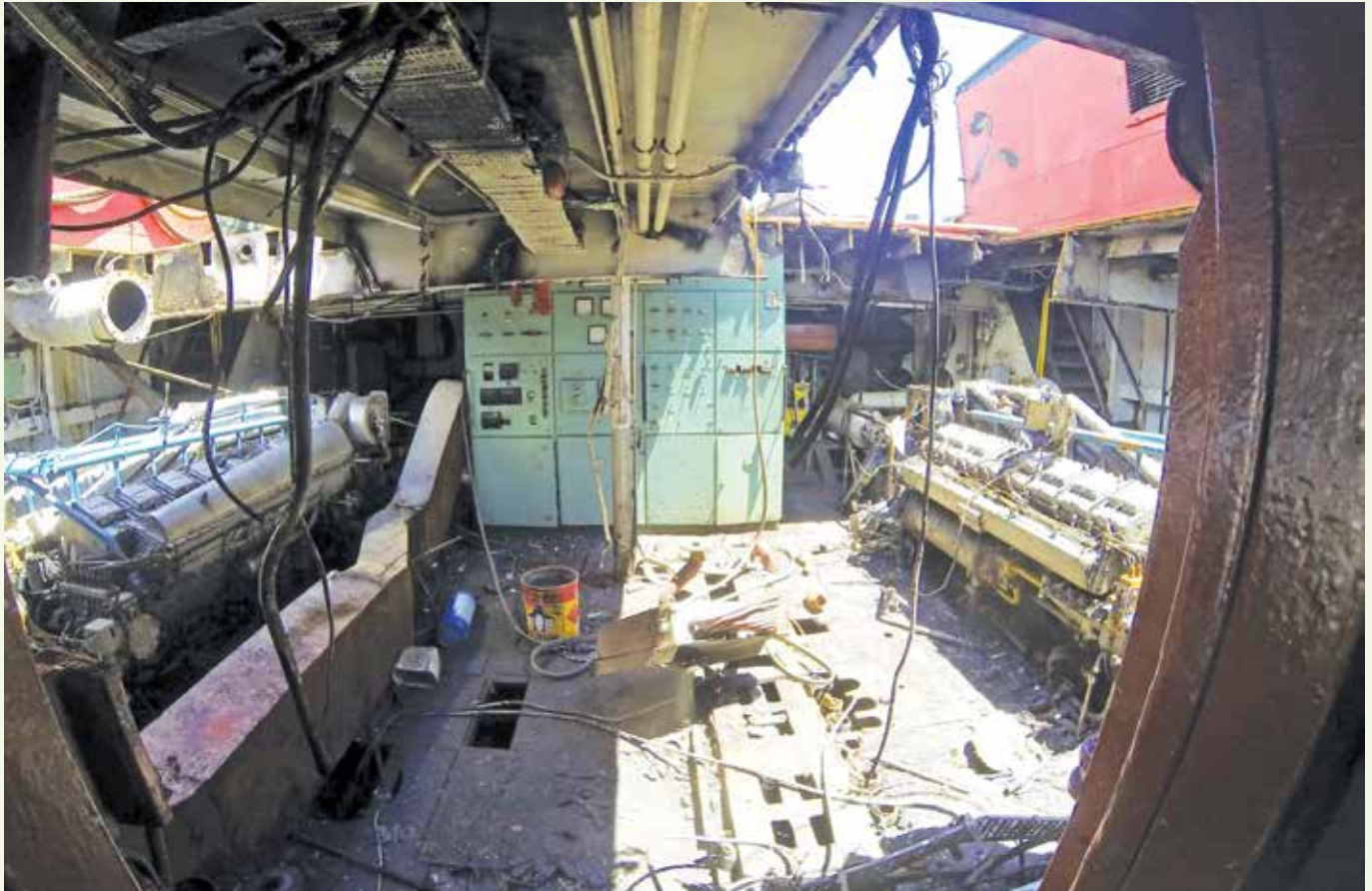
The engine room of the MPV Fish Eagle undergoing cleaning and preparation. Note how holes have been cut in the ceiling to allow the twin 16 cylinder engines to be removed via crane. These openings also act as comfortable entry points for penetrating wreck divers.
