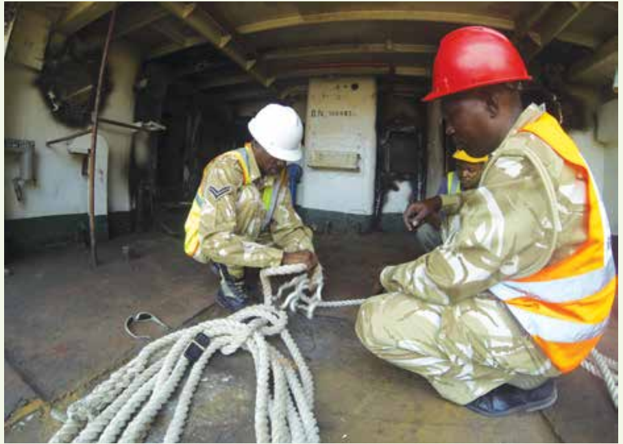
Top: The Kenya Wildlife Service preparing moorings which will be attached to the vessel. These moorings will be used to identify the site of the MPV Fish Eagle by dive operators enabling them to send divers to dive the artificial reef.
